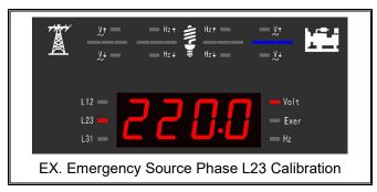
Step 4: Use a good quality voltmeter as a reference to calibrate the ATS-385 voltage reading to the desired phase.
