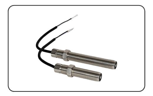
Is a measuring device for monitoring the speed of the driving force. When a ferromagnetic object (Usually the generator's flywheel gear) passes by the tip of the MPU, it produces a magnetic field and the MPU induced a voltage signal internally and the frequency of the voltage as the input to the speed control signal and accurately measure the prime mover speed.
