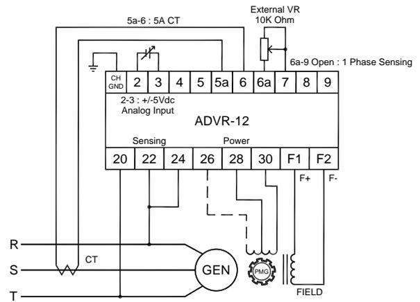
Figure 4 Single Phase Sensing PMG or Auxiliary Winding
