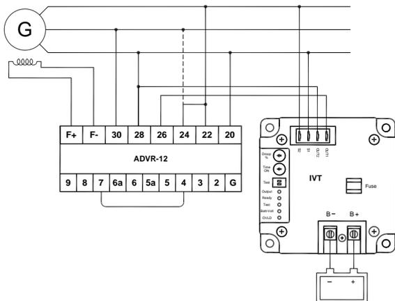
Figure 7 ADVR-12 & IVT-1260 / IVT-2460 Wiring Connection
