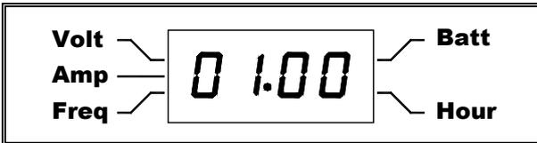
The first 2 digits represent the line number from 01 to 53, the last 2 digits stand the values for that line. You can change the value of the last 2 digits by using the UP and DOWN arrows following the table on (3.11)
