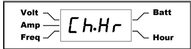
Now you can change the hour-meter by using the UP / DOWN arrows.
