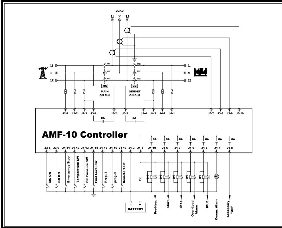
6.2.4 Single Phase Wiring Diagram
