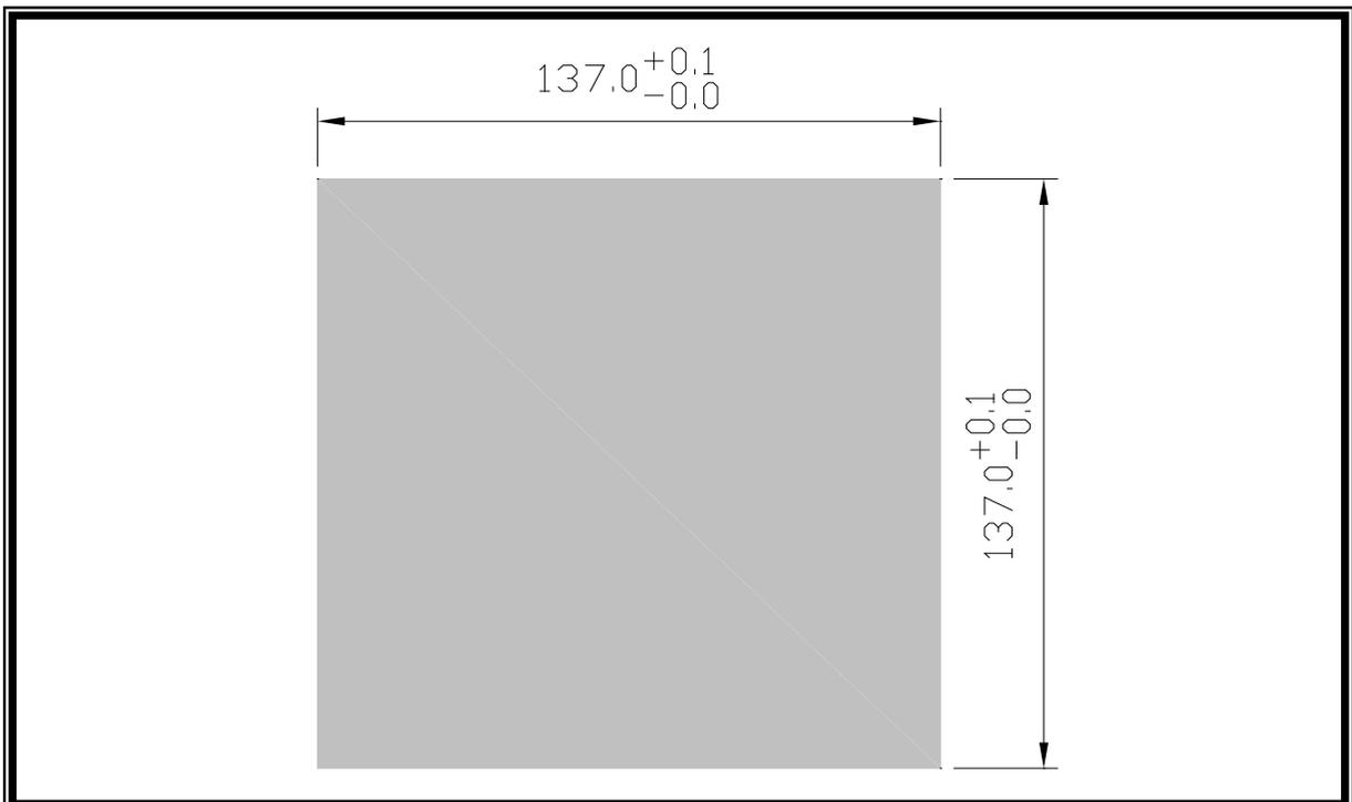
1.4 Unit Dimensions (Measurement : mm)
