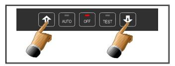
Step 6 : Press the "OFF" button to move to the next phase or until the word "End" appears on the screen. To exit hold the "OFF" button at any time for 4 sec.
