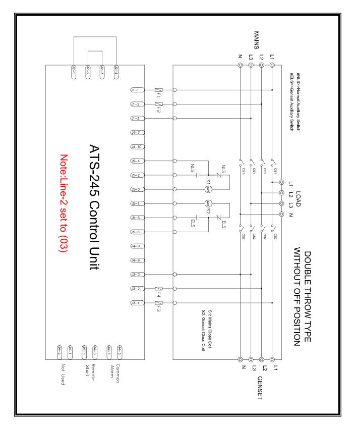
5.11 Double Throw Type ATS Without OFF Position Wiring Diagram (3P/4P) – With S1 & S2 Coils
