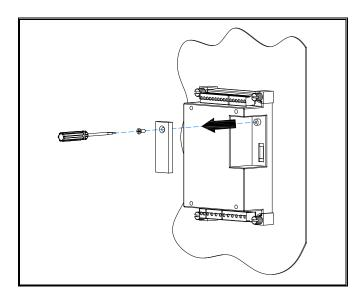
Step 2: Insert KCU-XX module into the slot and tighten the screw.
