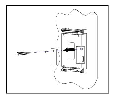
Step 2: Insert KCU-XX module into the slot and tighten the screw.
