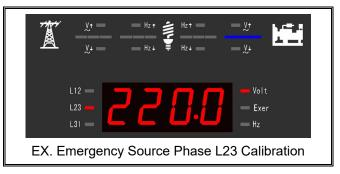
Step 4: Use a good quality voltmeter as a reference to calibrate the ATS-22A voltage reading to the desired phase.
