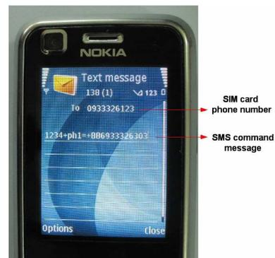
Step 5 : After completing Step 4, send out the text message.
