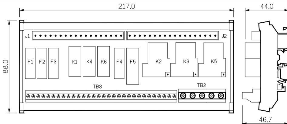
鋁軌(DIN Rail)規格: 3.5 x 7.5 mm
