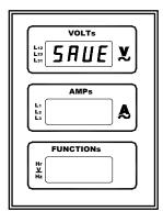
If the buttons are left untouched for 10 seconds, the operation terminates showing (END) on the screen and the control turning OFF and any modification made to the hour meter will not be recorded.
