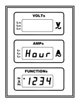
Press the UP and DOWN buttons to change the hours. By pressing and holding, you can speed up the process. When the setting is completed, press the (PEN) button for 4 seconds until (SAVE) appears on the screen.
