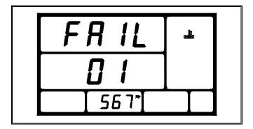
The **(FAIL)** and **(01)** represent the event log screen (is the memory lines 1 to 15), the **(567 Hr)** represents the hour when the failure occurred and the Overheat icon represents the cause of the failure.
