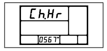
Now press **(UP Arrow)** or **(Down Arrow)** button to change the hour reading. By holding down the button you increase the scrolling speed.
