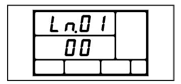
(Ln.01) indicates Line.1, and (00) representing the entered value. You press (**UP Arrow**) or (**Down Arrow**) to change the value. Each time you press the Pen Button we move to the next Line. If the setting is left unattended for 30 seconds or if the last Line 68 is reached the word **END** indicates that you finished and all modified values are saved.
