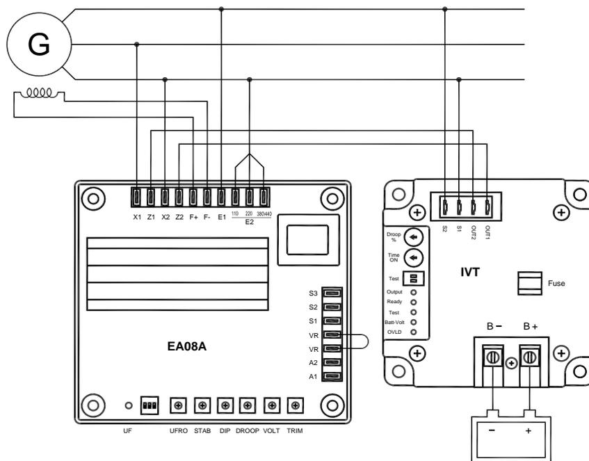
Figure 3 IVT-1260 / IVT-2460 & EA08A Wiring Connection
