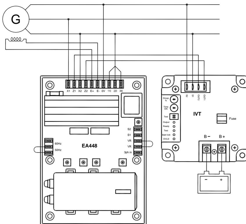
Figure 4 IVT-1260 / IVT-2460 & EA448 Wiring Connection
