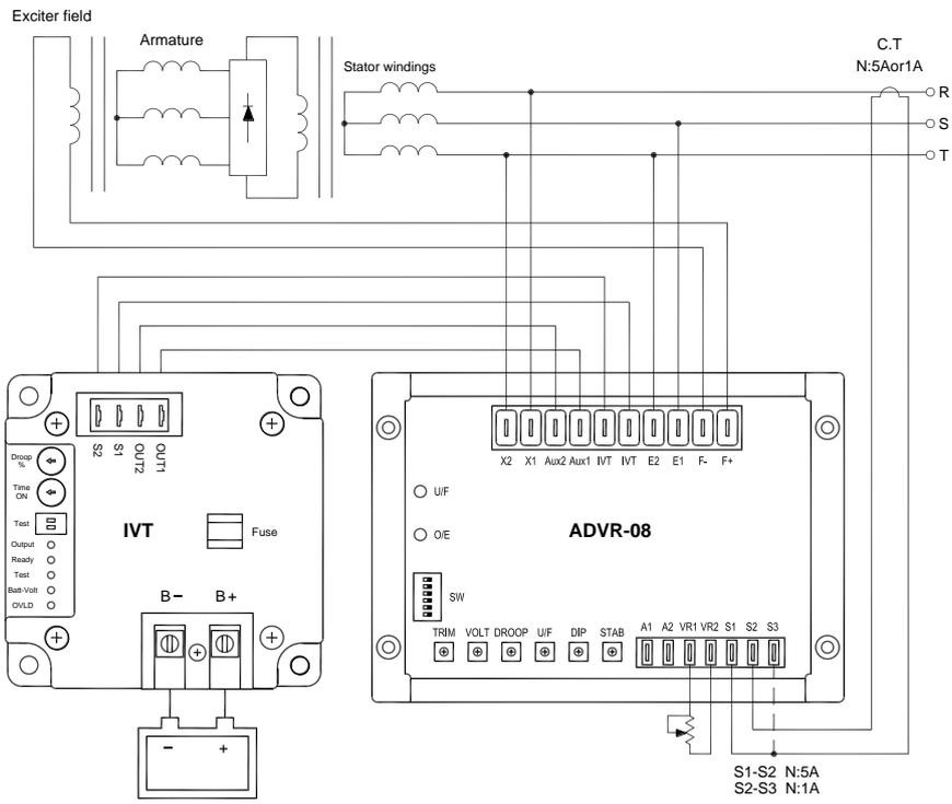
Figure 5 IVT-1260 / IVT-2460 & ADVR-08 Wiring Connection
