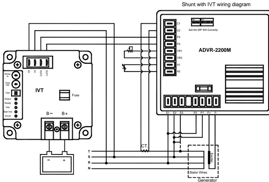
Figure 7 IVT-1260 / IVT-2460 & ADVR-2200M Wiring Connection
