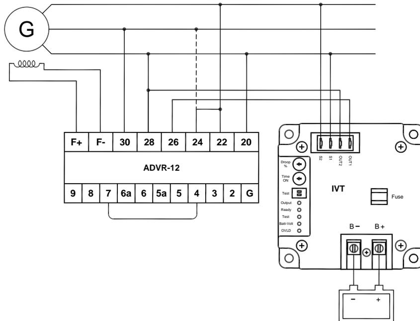
Figure 6 IVT-1260 / IVT-2460 & ADVR-12 Wiring Connection
