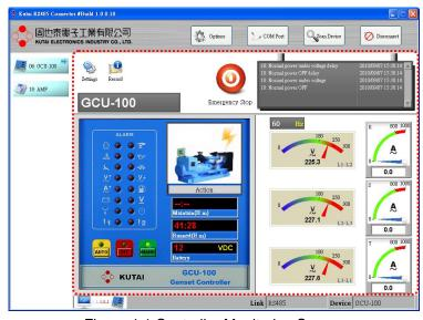
Figure 4-1 Controller Monitoring Screen
