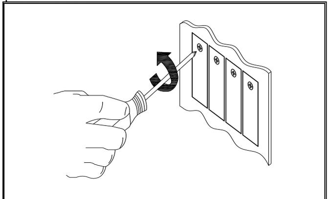
Step 2 : Insert KCU-41 module into the controller's expansion slot.
