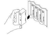
**Step 2:** Insert the KCU module into the controller's expansion slot
