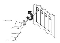
**Step 1:** Remove the expansion slot cover from the controller
